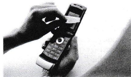
NovaCryl removable PSAs can be used in protective films for consumer electronic display applications.
